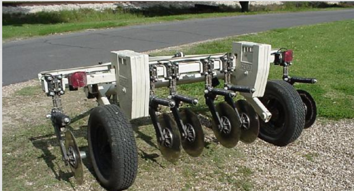
Veris® 3100 Soil EC Mapping System
