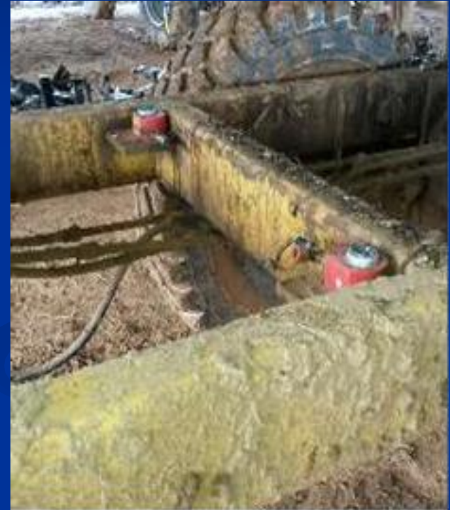
Figure 3: Hydraulic load cells mounted in trailer frame.
