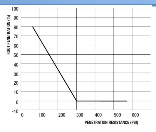
The penetrometer simulates root growth. Root growth decreases linearly with increasing penetration resistance, until practically stopping above 300 psi. Remember, however, that roots may still penetrate soil with a penetration resistance greater than 300 psi if natural cracks and pores are present.
