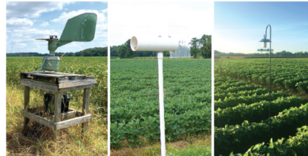
Figure 1: Spore traps placed around soybean fields in Louisiana include the Burkard spore trap, wind vane spore trap and garden motor spore trap. These are used to monitor peaks of spores of the pathogens causing Cercospora leaf blight of soybean. Photos by Sara Thomas-Sharma
